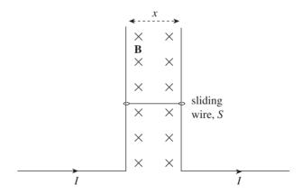
The mass of the sliding wire, S, is m. If the sliding wire S crosses a region that contains a uniform magnetic field  $\mathbf{B}$ , how much current must be carried by the wire to keep S from sliding down (due to its weight)?
